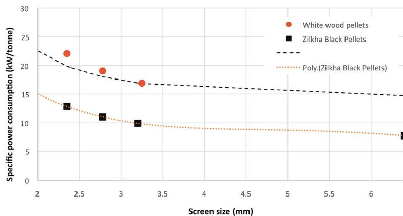
Figure 6. Specific power consumption in a hammer mill plotted vs mill screen size.
