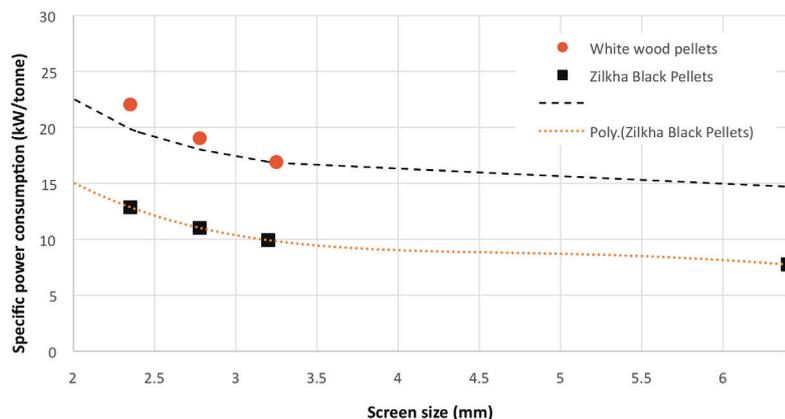
Figure 6. Specific power consumption in a hammer mill plotted vs mill screen size.
