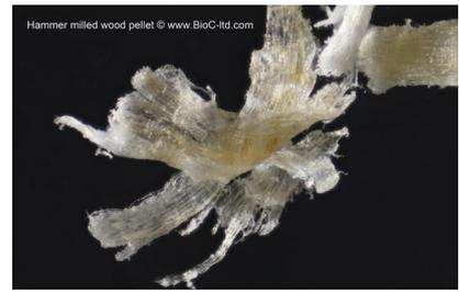
Figure 3. Particle from wood pellets milled in a hammer mill.
