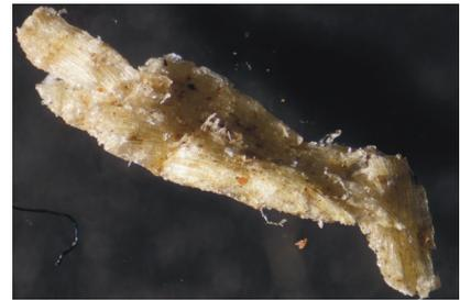
Figure 4. Particle from wood pellets milled in a vertical spindle mill.
