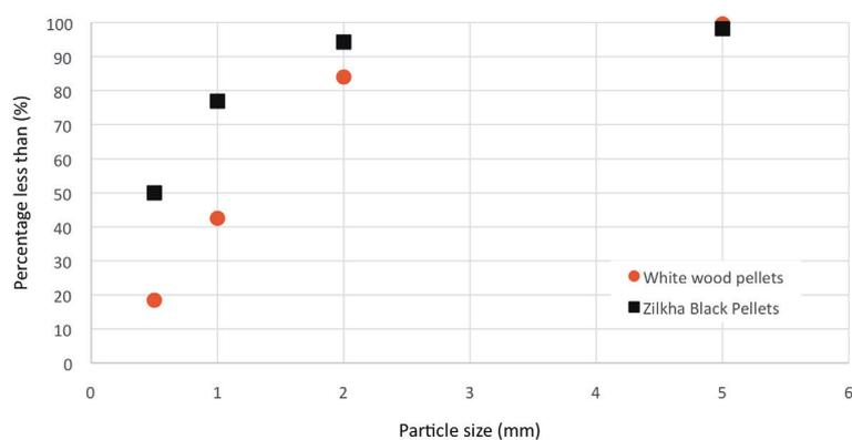
Figure 7. Size distribution of the mill product from a hammer mill with 6.4 mm screens.
